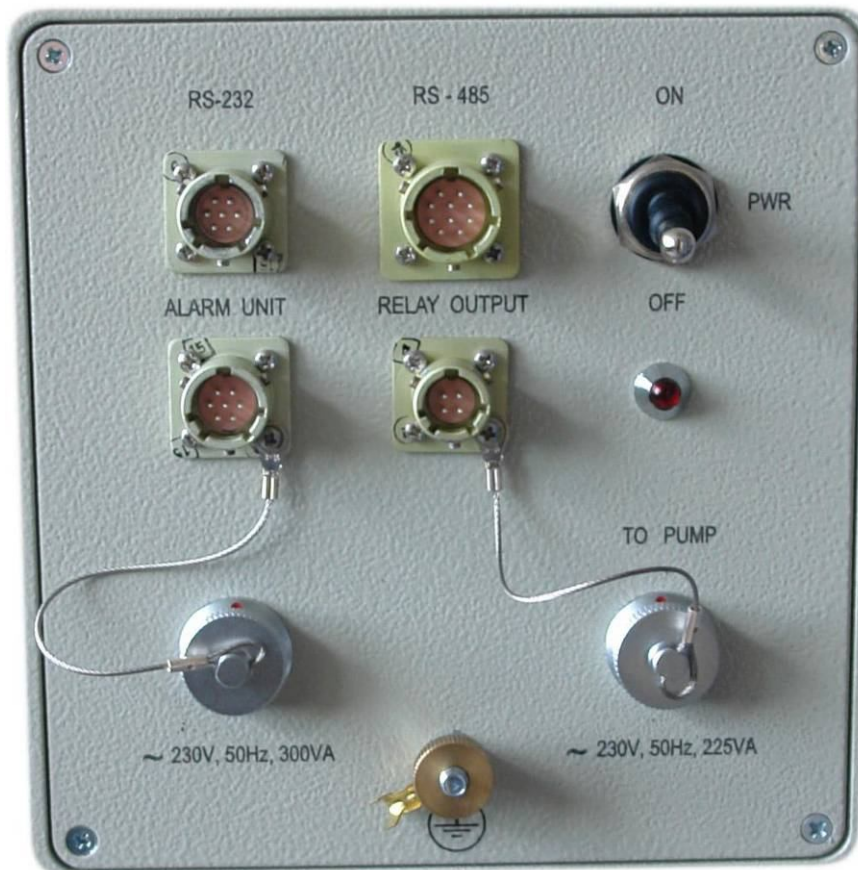
Figure 1.2 – External interface connectors
