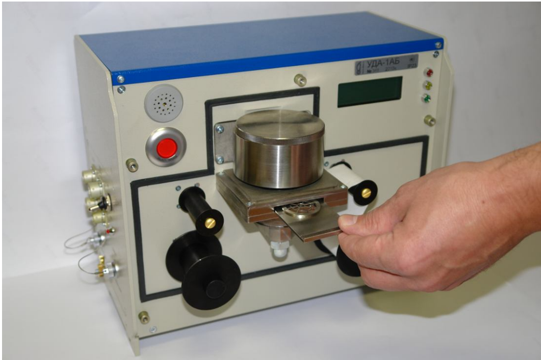
Figure 4.2 – Removal of the filter screen
