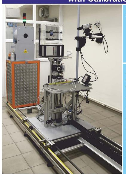
Reference gamma beam irradiator with calibration bench is designed to simulate and transmit air kerma, exposure dose, individual dose equivalent and dose equivalent units and their respective rates into working standards and measurement instruments during verification, calibration and test procedures.
