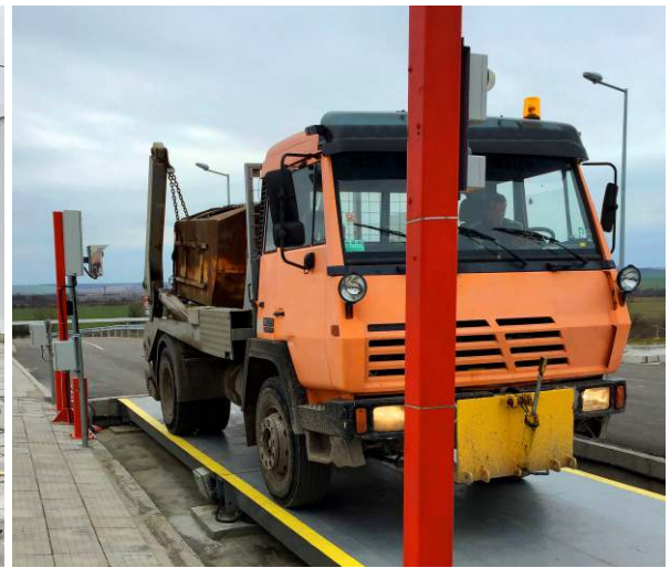
Version of vehicle radiation monitor with the following configuration: BDRM-05 (8 units), BDKN-05 (8 units)
